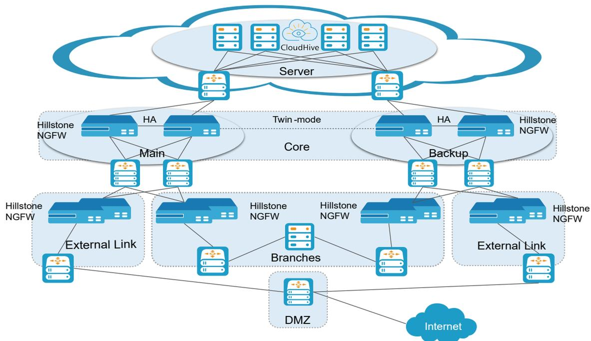
across data centers to maintain full security for all redundant data center traffic flow. With Hillstone's unique Twin-mode firewall solution, the E-Series firewalls automatically synchronize configuration and session information among the high-availability pairs. For instance, in a virtual environment running VMware, this synchronization ensures uninterrupted service during vMotion between data centers
